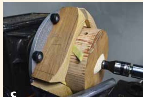
Shims are used to adjust the position while centering the blank. The jaw's buttons visible here were used only as an aid in setting up each of the four wasteblocks, providing a reference point until the blocks were mounted with screws. The buttons are not involved in holding the wooden extensions in place. Note the protective scrap wood between the live center and the blank. The tailstock can be removed to allow access for light, final shaping cuts.
