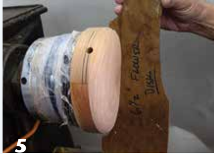
5 A hardboard template used on both faces ensures similar opposing curves.
