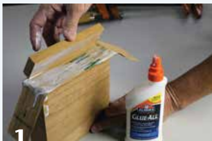
1 Glue a temporary wasteblock onto the vase blank using a paper glue joint.
