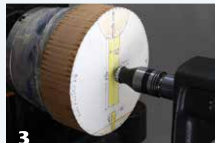
3 After bandsawing the blank round, center it using the point of the tailstock live center for alignment.
