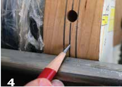
4 Layout lines on the blank's outer edge aid in the symmetrical shaping of the two faces.
