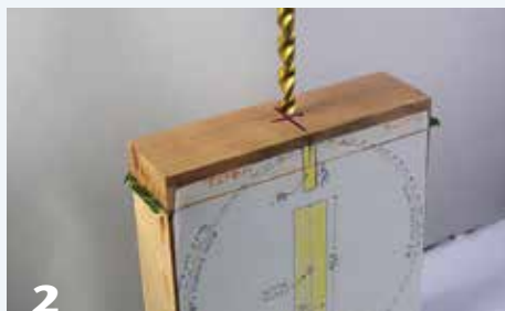
2 Mount the full-sized drawing onto the blank and drill through the wasteblock for later mounting on a screw chuck.
