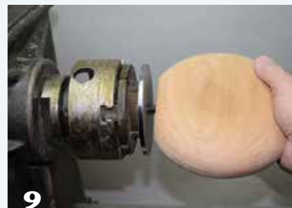
9 Mount the disk on the screw chuck, establishing a new axis for turning. Note the metal stabilizer/spacer, which provides a flat surface on which the disk can seat.
