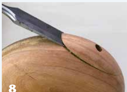
8 Use a chisel to remove the wasteblock, exposing a flat, which is critical to safe mounting on a screw chuck.
