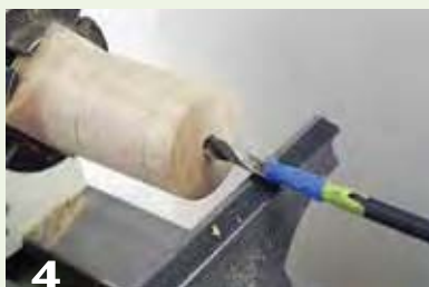
4 Drill a hole into the center of the bell to make hollowing easier.
