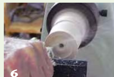
6 Hollow the interior of the bell. You are cutting endgrain, so cut from the center out.
