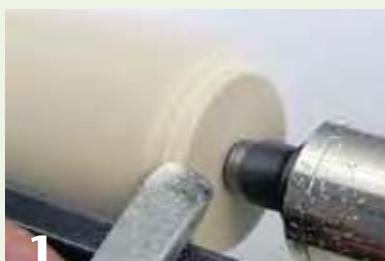
1 Form the tenon with a peeling cut using a skew chisel.
