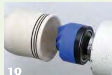
10 Masking tape around the live center will help support the bell as you part it off.
