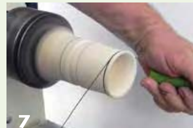
7 To decorate the bell, burn lines using a wire, held by wood handles.
