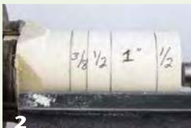
2 Mark the blank with the bell's key dimensions. Use these dimensions to determine the depth to drill the hole.
