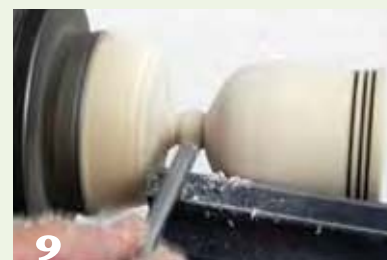
9 Take clean cuts, working from the shoulder to the button, to create a crisp transition between the bell's shoulder and the button.
