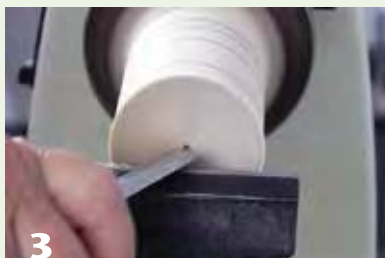
3 Cut a small indentation to mark the center. Use the long point of a skew chisel.
