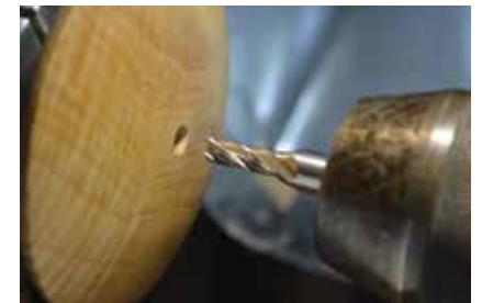
Without the centerpoint of a Forstner or bradpoint bit, a milling cutter drills a deeper stopped hole with a flat bottom.
