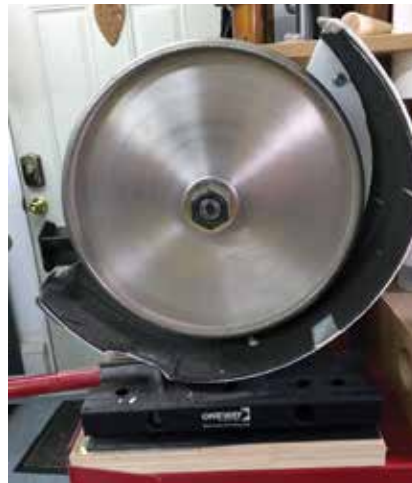
A custom magnet shroud does a great job of capturing grinding dust from CBN wheels.
